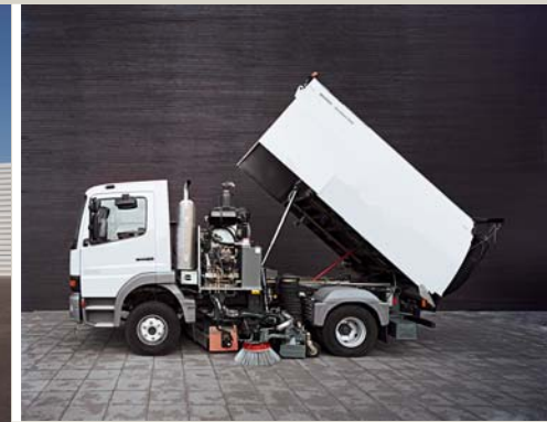
Truck mounted sweepers
